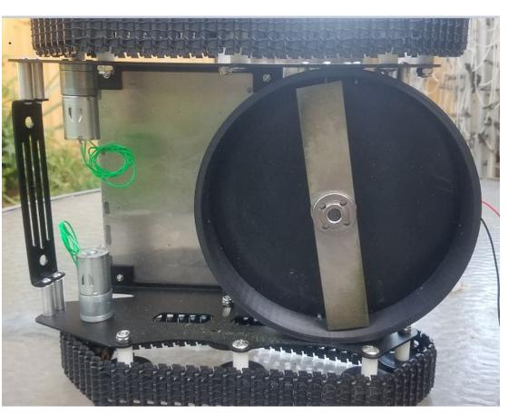
Installed cutter blade shroud
