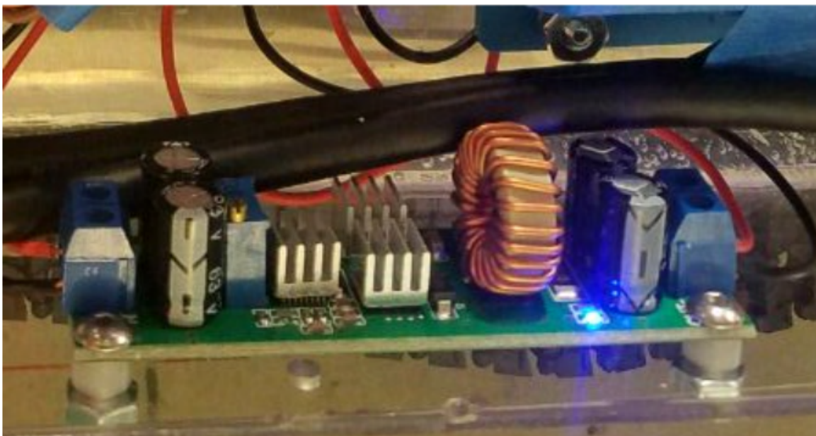
Figure 2.12 DC to DC Step Down Voltage Regulator
