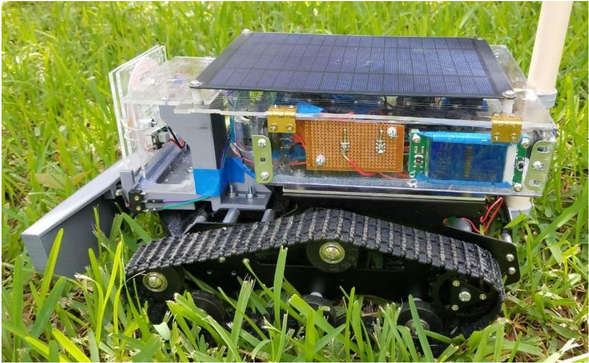
Figure 3.25 Grass height interfering with mower turning
